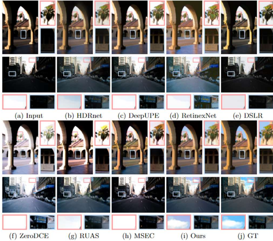
Fig. 8: Visual comparison of over-/under-exposed images from our dataset. Our model reconstructs the details in the over-exposed regions (sky and tower) as well as the under-exposed regions (wall and door).
