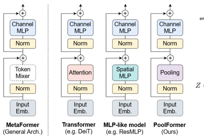
embedding dimension embedding tokens  $X = \text{InputEmb}(I), \ X \in \mathbb{R}^{N \times C}$ sub-block 1 Y = TokenMixer(Norm(X)) + X,sub-block 2  $Z = \widehat{\sigma}(\text{Norm}(Y)W_1)W_2 + Y,$ **Activation Function**  $W_1 \in \mathbb{R}^{C \times rC}$  $W_2 \in \mathbb{R}^{rC \times C}$
